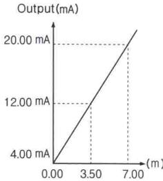
This function can change the 4~20mA value as the output scale.
