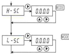
This Function changes and sets the display value according to scale and input range.
