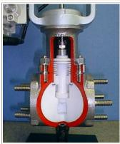
Type T-8210 Acid-Proof Control Valve starting with chemicals is Gland packingless structure control valve which is suitable for control of all kinds of acid and Alkali fluid. By using small size high output Multi-spring type Actuator with positioner, it is extremely compact control valve.
